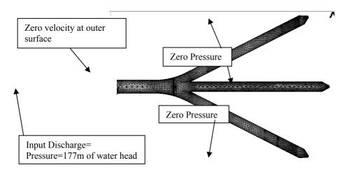
Fig 3 Boundary condition for most efficient trifurcation control volume
