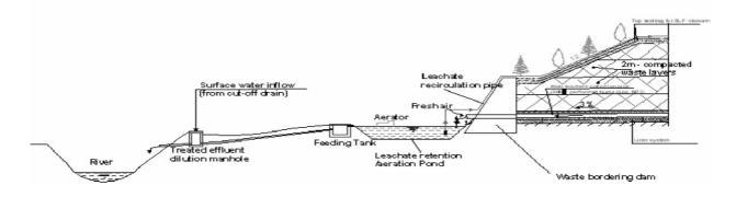
Fig 4 Leachate treatment plant in Sisdol landfill Site.
