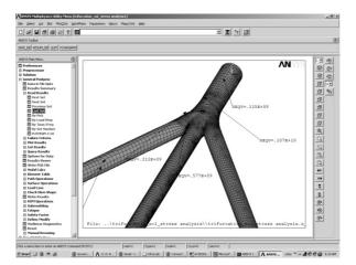
Fig 13 Mesh generation of manifold with shell 181 element, for stress analysis.
