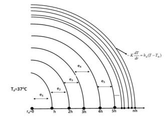
Fig 1 Finite Element Discretisation Mesh.
