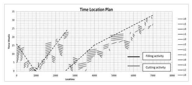
Fig 3 Model-generated time-location plans of a 7 km road project
