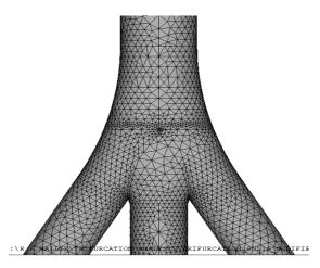
Fig 2 Tetrahedral meshing of fluid control volume near junction
