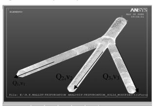
Fig 1 Ansys meshing of the trifurcation fluid control volume
