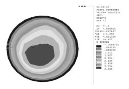
Fig 10 Velocity distribution in sections 5-5
