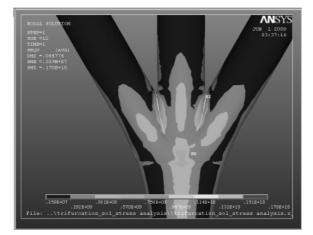
Fig 14 Von-misses stress distribution, showing stress concentration near junction. Stress near junction exceeds yield strength of mild steel for water pressure below normal water pressure
