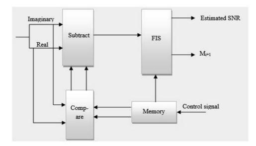
Fig 2: Fuzzy Logic SNR Estimation and Modulation Control
