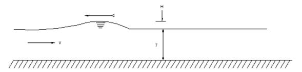
Fig 1 Propagation of low wave in channel
