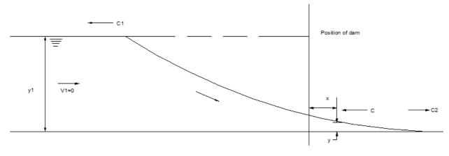
Fig 12 Dam Break illustration
